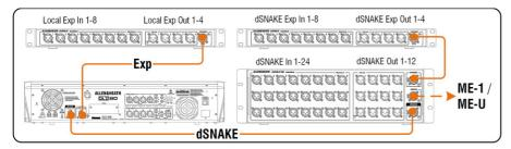
GLD + AR2412 + 2x AR84 Expanded AR system 48 in, 30 out 40 remote mic inputs
