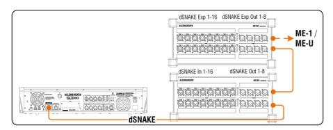
GLD + 2x AB168 Two digital stage boxes 40 in, 26 out 32 remote mic inputs
