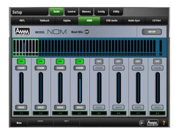
NOM (Number of Open Mics) mode evolved from the AMM developed for the Allen & Heath IDR8 installed sound processor, NOM mode acts as a gate, turning an input on when a threshold is passed. The level adjustment for each open input is equal and depends on the number of microphones open and the NOM attenuation parameter which sets the amount of attenuation applied for every doubling of open microphones.
