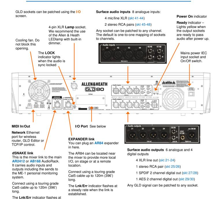
I/O Port options for system linking, expansion, recording and audio networking using one of the option cards available from Allen & Heath. 64 channel bi-directional 48kHz audio.
