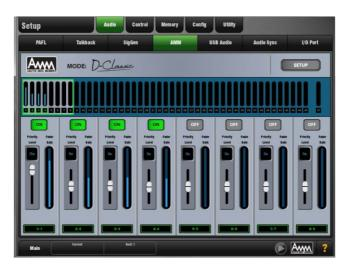
Unlike NOM mode which uses gating and fixed gain attenuation, D-Classic uses a 'constant gain sharing' algorithm to dynamically adjust the gain for each mic proportional to its input level. Louder signals will receive more gain in the mix.
