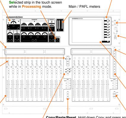
USB ports For transferring Show files, Libraries and event logs, stereo playback and recording to USB, and for updating
