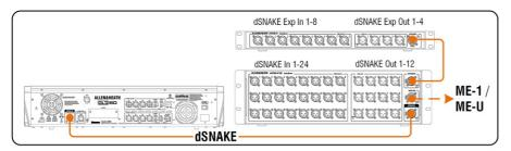
GLD + AR2412 + AR84 Expanded AR system 40 in, 26 out 32 remote mic inputs
