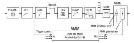
The AMM takes control by first setting each assigned channel fader to '0' (0dB unity gain), thus effectively passing the signal unaffected through the fader, and then using its own post-fade gain element to make its automatic adjustments. It is typical to leave the faders at '0', but they can be adjusted if the engineer wishes to make additional post AMM level changes manually to adjust the relative balance between mics in the mix.
